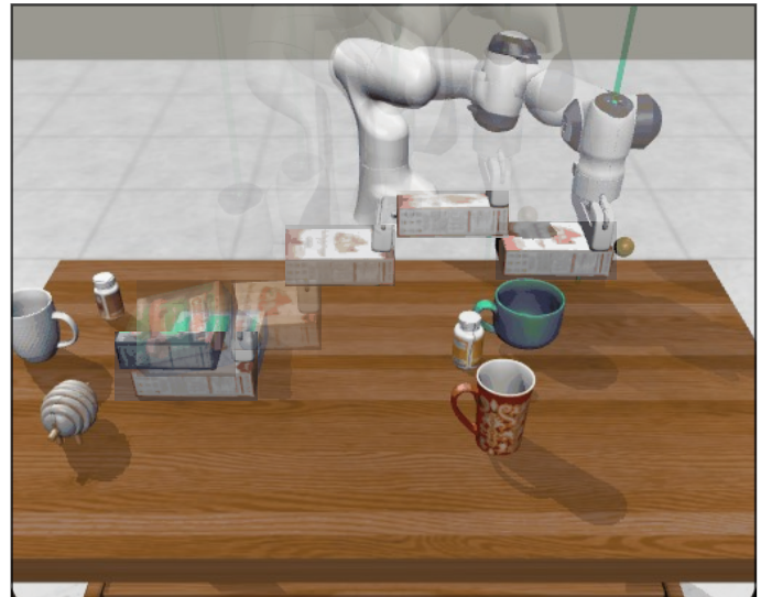
Figure 1: Dynamic manipulation task: The robot dynamically, but carefully, slides a target object from under another object, and moves it to a goal region while avoiding safety-critical objects on a cluttered table.
